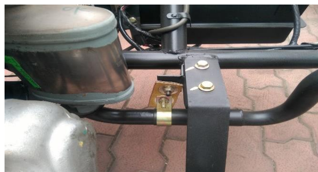
Fig. 15. Catalytic converter mounting position After
