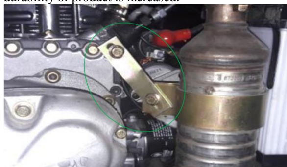
Fig. 14. Catalytic converter mounting position before
