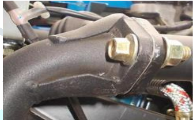
Fig. 17. Exhaust flange mounting with reinforcement
