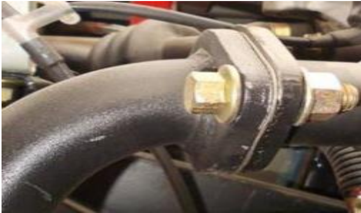
Fig. 16. Exhaust flange mounting without reinforcement
