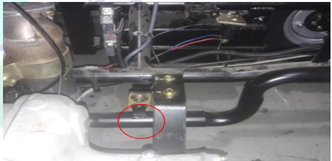
Fig. 13. After modification mounting of the exhaust pipe
