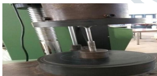
Fig.5 Compaction under CTM
