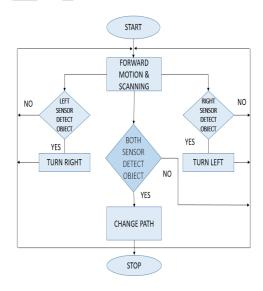
Fig 1.1: Principle of motion of robot car
