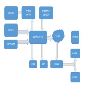
Fig 1: Block diagram of rescue assistant robot
