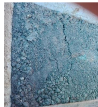
Fig. 9: Initial failure of slope at 133 mm/h rainfall intensity for slope angle 45^\circ
