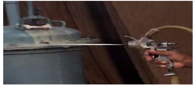
Fig 2: 500g of latex is spreaded
