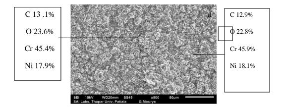
Fig 1 SEM/EDAX analysis of characterization of coated substrates of the boiler steel was:
