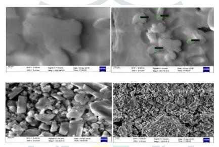
Fig.5. FESEM micrograph of nanosilica
