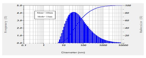
Fig.7. DLS analysis of nanosilica particles
