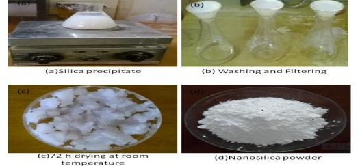
Fig.2.Synthesis of nanosilica by precipitation method
