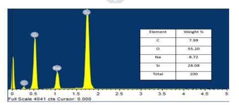
Fig.6. EDX of nanosilica particles.
