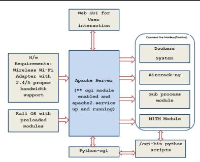
Figure 2. Architecture Diagram of DEADSEC
