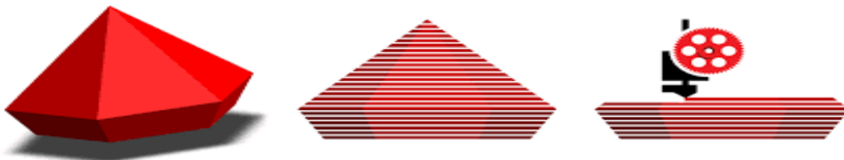
Figure 6.2 Slicing of a 3D model
