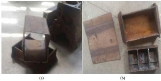
Figure 6. (a) Steel plate before bending, punch and die; (b) The folded plate.
