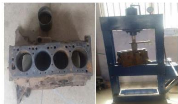
Figure 4. (a) Cylinder engine block before pressing sleeve; (b) Cylinder engine block after the pressing of sleeve.
