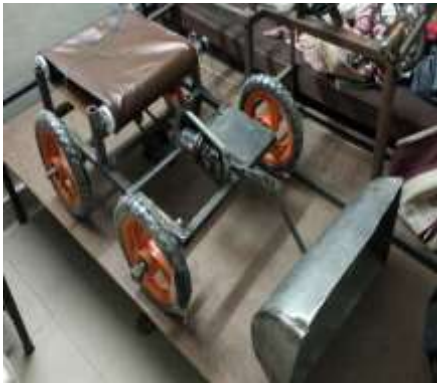
Fig 3: Final Assembly of Sand Collector
