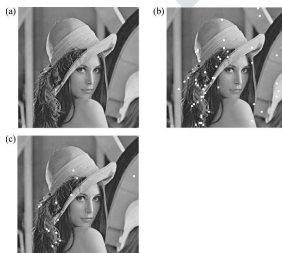
Figure 4: (a) Decrypted image using content owner's key. (b) Blocks of incorrect recovery of Zhang's method. (c) Blocks of incorrect recovery of the proposed method.
