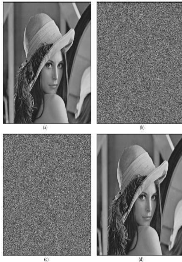
Figure 6 (a) Original Image (b) Encrypted Image (c) Encrypted image containing embedded data with embedding rate with 0.017 bpp (d) directly decrypted version with PSNR 39.0 dB
