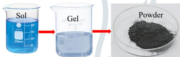
Fig. 1: Pictorial representation of different phases of sol-gel process.
