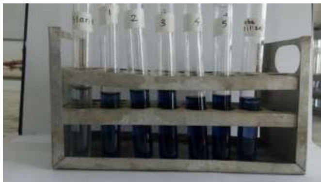
Fig. 22: Protein estimation by Lowry’s method
