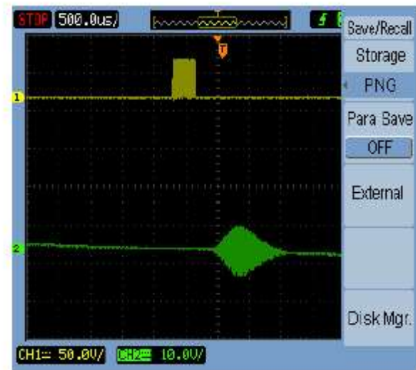
Figure 4 Transmitted (CH1) and Received signal(CH2) on CRO
