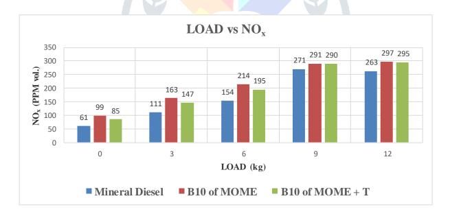
Figure: Plot shows the variation of NO<sub>x</sub> emission with Load of Blends
