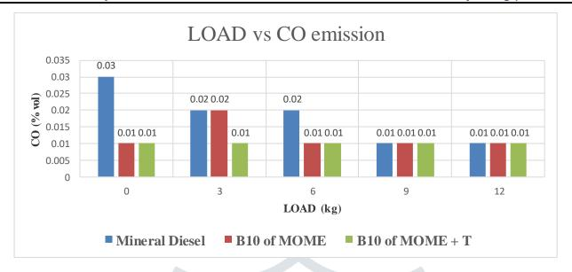
Figure: Plot shows the variation of CO emission with Load of Blends
