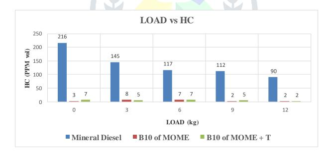
Figure: Plot shows the variation of HC emission with Load of Blends
