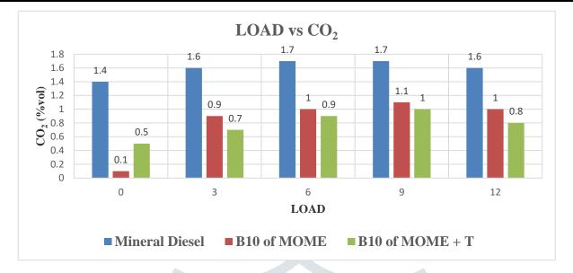
Figure: Plot shows the variation of CO<sub>2</sub> emission with Load of Blends
