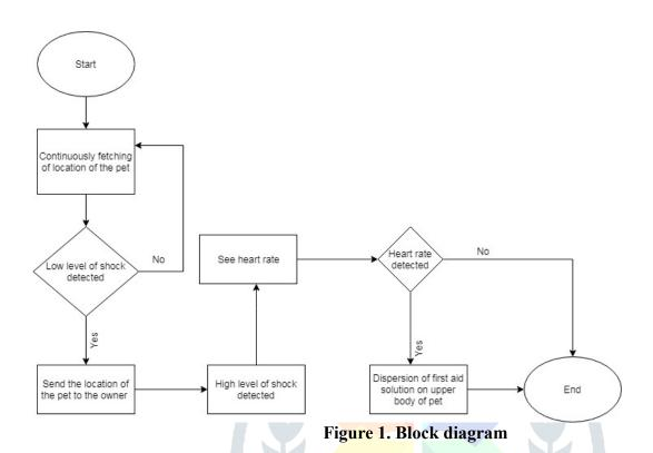
The location tracking system continuously fetches location of the pet. The shock sensor senses low level shock and high-level shock.
