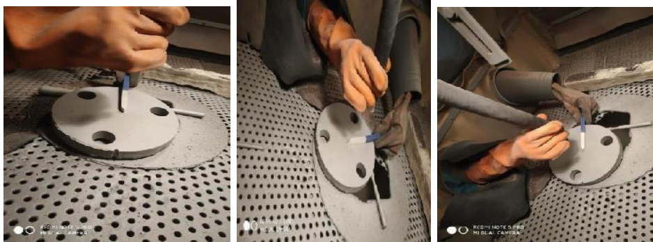
Figure4-6:Sand blasting for CuttingTool
