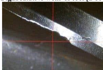
Figure1.2:Excessive wear of a tool [2]
