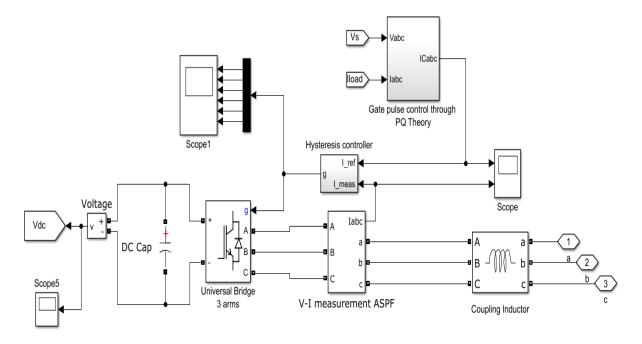
Fig. 6: subsystem of active shunt filter
