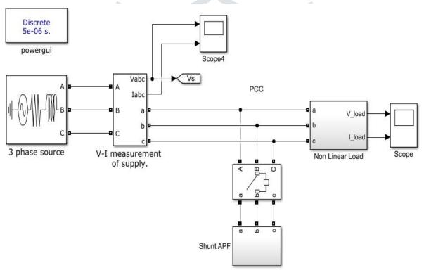
Fig. 5: MATLAB simulation diagram of ASF for p-q Theory
