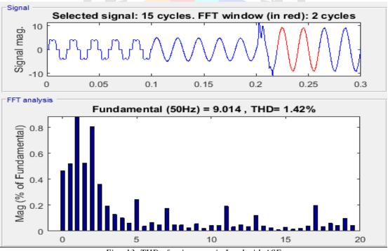
Fig. 13: THD after increase in Load with ASF
