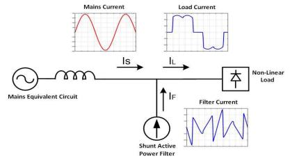
Fig. 1: Basic diagram of ASF
