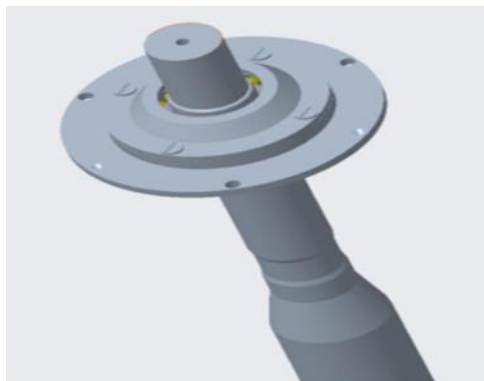
Fig 9: Assembly of agitator shaft with bearing
