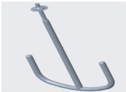
Fig 8: Assembly of agitator shaft
