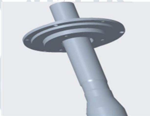
Fig 10: Assembly of agitator shaft and bearing housing
