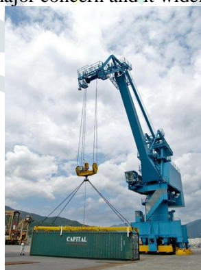
Figure 1 Level Luffing Crane
