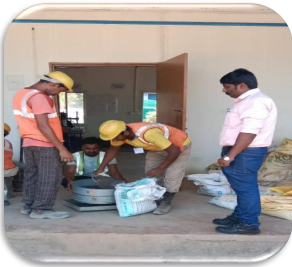
Recycled / Milled aggregate gradation and testing in progress Fig No.9
