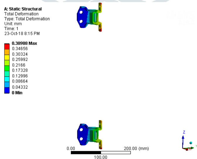
Fig8: Displacement result for Door Hinge
