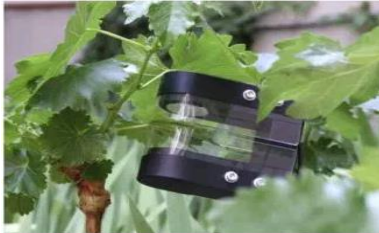
Figure 1 : Specially designed pair of air-coupled transducers mounted on an U-shaped holder to take NC-RUS measurements in Vitis vinifera leaves.
