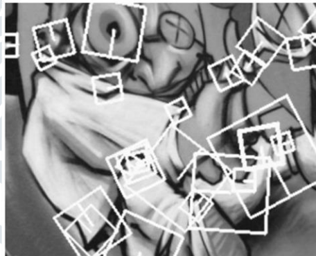
Fig. 8: Detail of the Graffiti scene showing the size of the oriented descriptor window at different scales.
