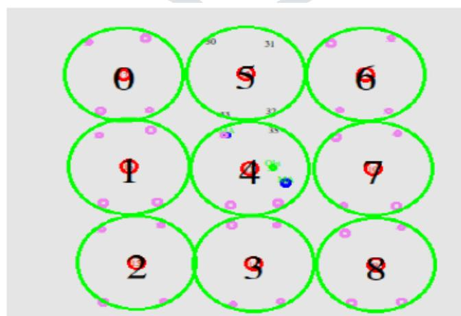
Fig 4.4 Detouring of Anchor Node due to the presence of obstacle in Anchor node trajectory
