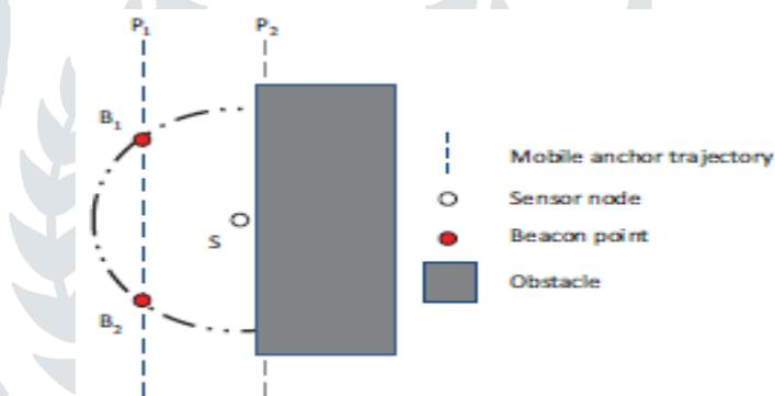
Fig 3.3 Impact of Obstacle in the Mobile Anchor trajectory
