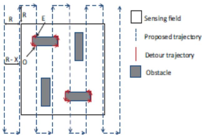
Fig 3.4 Obstacle resistant trajectory of mobile anchor node.
