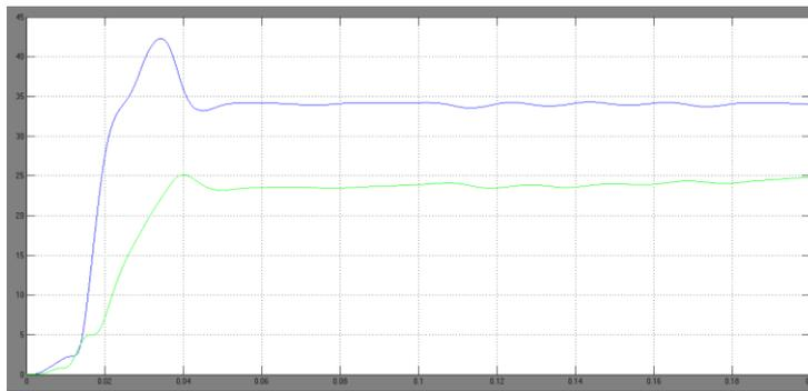
Fig. 4.10 Power flow with LC ladder ref P-Q<sub>rms</sub>
