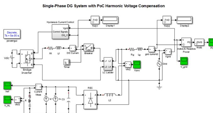
Fig. 4.5 Simulation Circuit of PoC harmonic Voltage mitigation
