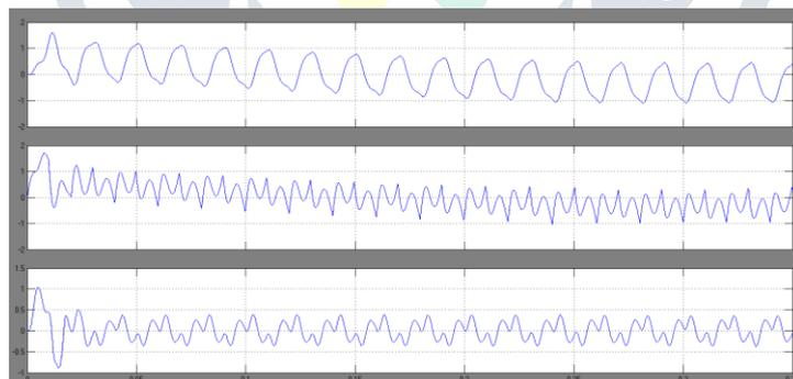
Fig. 4.2 Performance of DG unit local load current harmonic compensation (a) grid current, (b) DG current, (c) local current
