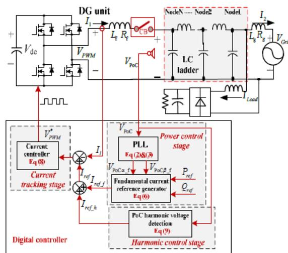
Fig. 2.2 DG unit with PoC harmonic voltage mitigation capability
