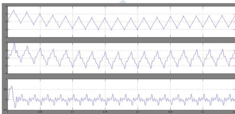
Fig. 4.4 DG unit during feeder resonance voltage (a) grid current, (b) DG current, (c) local current
