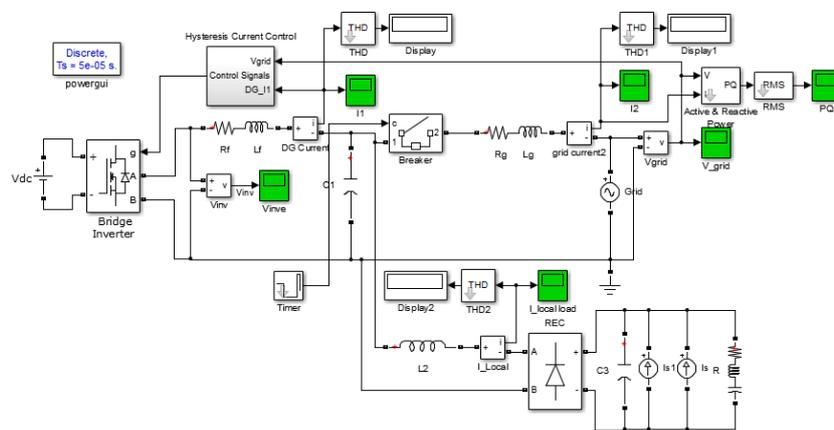
Fig. 4.1 Simulation circuit of Local Load harmonic current compensation
