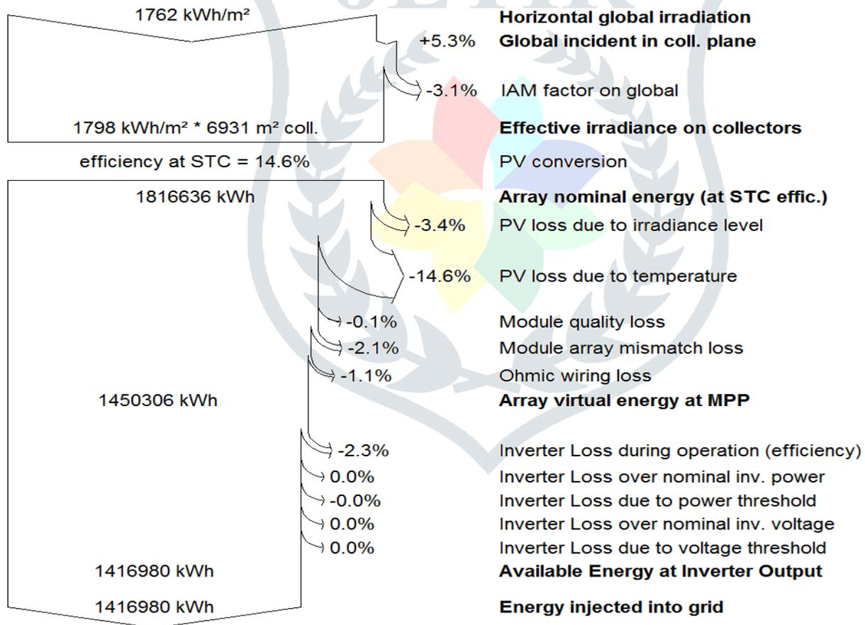
Figure 4 System Loss Diagram
