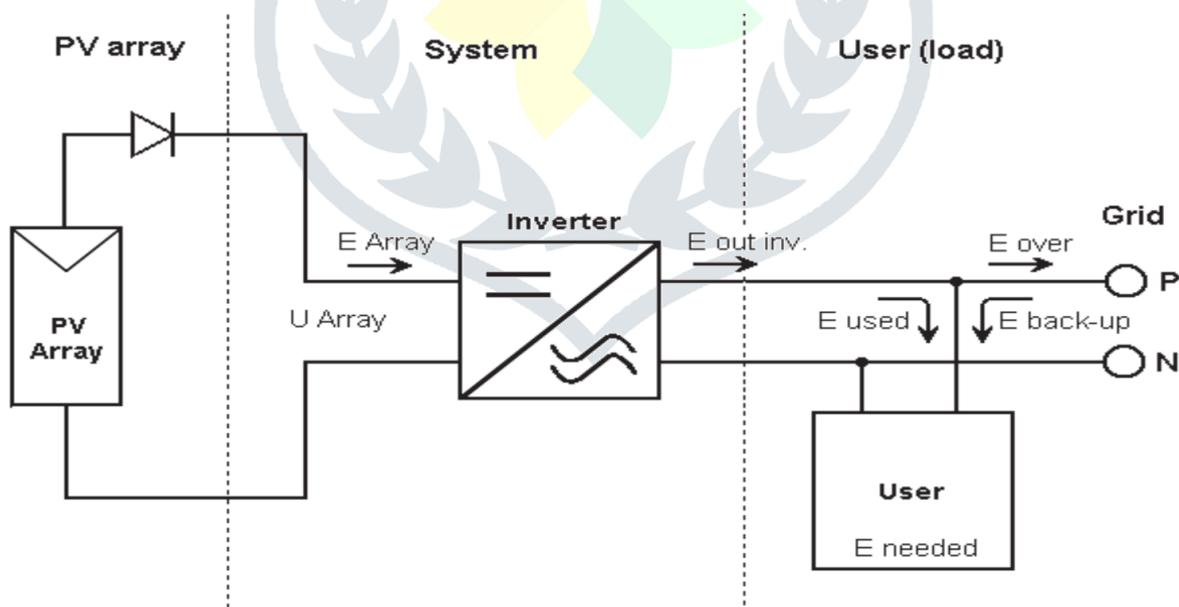
Figure 1 Grid connected PV system
