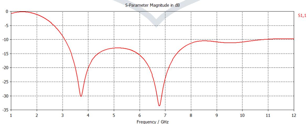
Figure 2 S<sub>11</sub> vs Frequency graph RETURN LOSS S<sub>11</sub> RESULT
