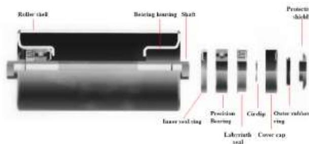
Fig.3.2.Parts of roller
