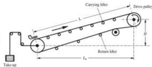
Fig.3.1.Principle working of belt conveyor
