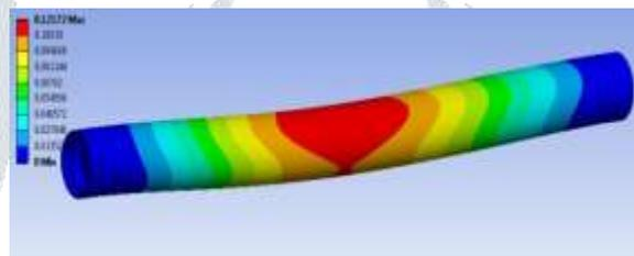
Fig.7.1. Deformation in new roller
