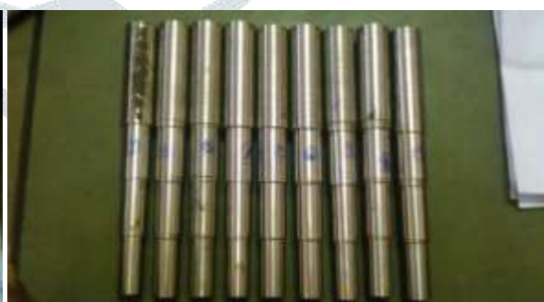
Image 3.3 round bars after turning
