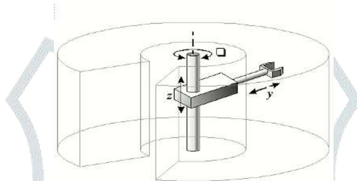
**Fig. 2. A 3-DOF cylindrical arm configuration and its workspace [4].**
