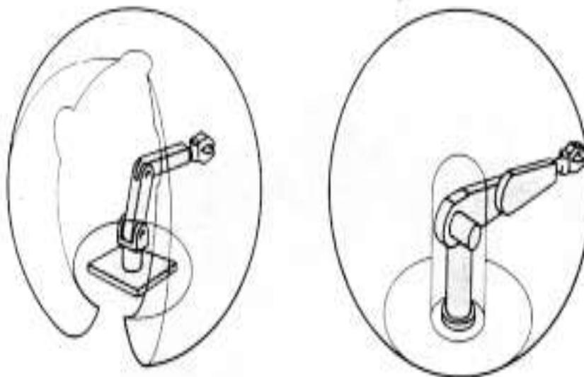
Fig. 4. A 3-DOF articulated arm configuration and its workspace [4].
