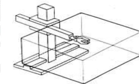
**Fig. 1. A 3-DOF Cartesian arm configuration and its workspace [4].**
