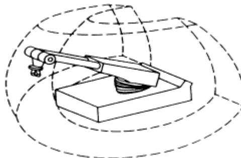
**Fig. 3. A 3-DOF polar arm configuration and its workspace [4].**
