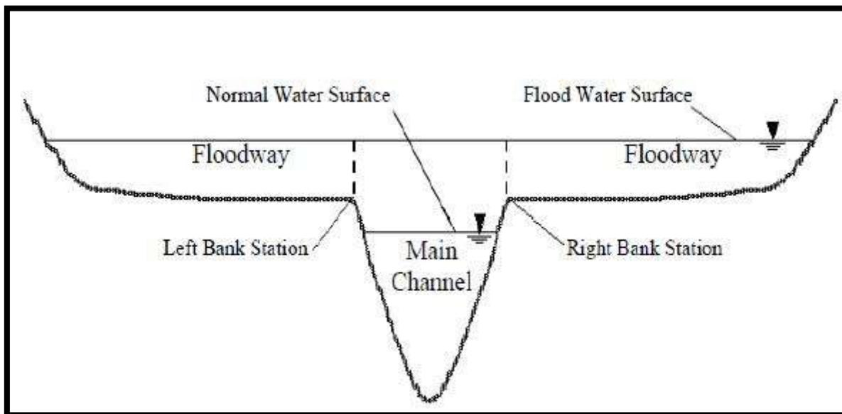
Figure 6 - Schematic daigram of stream channel
