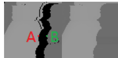
Fig. 3: (a) Warped depth map; (b) Filled depth map using depth based extrapolation [2]
