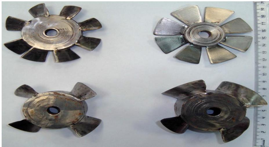
Fig.5 Working rotors R1, R2, R3, and R4 for the model propeller hydro turbine
