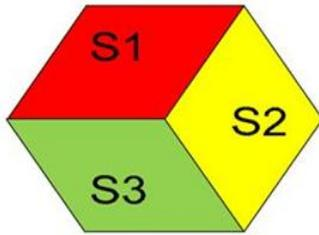
Figure 4. 120 degree Cell Sectoring
