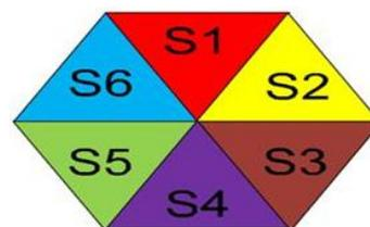
Figure 3. 60 degree Cell Sectoring
