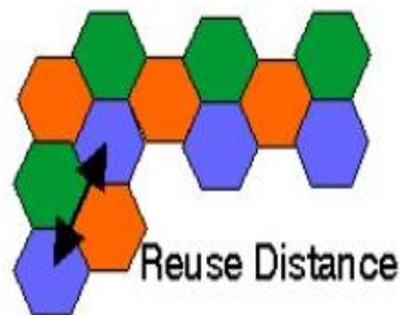
Figure 1. Frequency reuse
