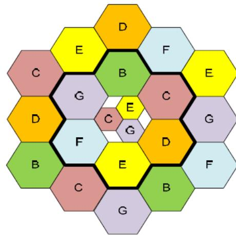
Figure 2. Cell Splitting
