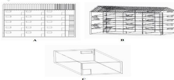
Fig -2: (A) Geometry of the cool storage, (B) Isometric view of the cool storage and (C) Experimental setup room geometry
