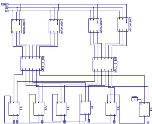
Fig 4- Direct digital synthesizer
