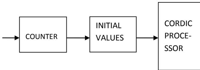
Fig 2- Direct Digital Synthesizer
