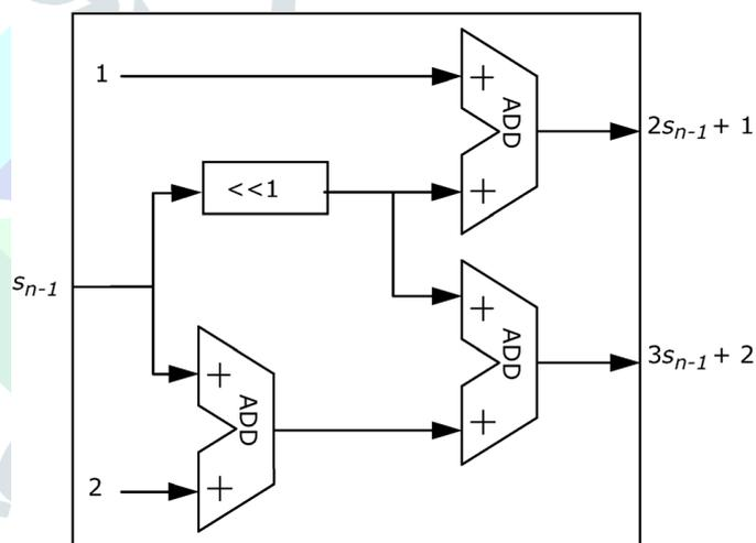
**Fig 1-** Adds and shift operation in CORDIC
