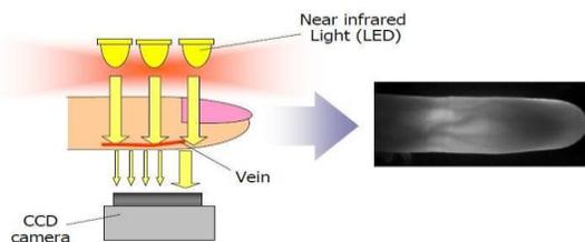
**Figure 1. Finger vein pattern captured by camera**
