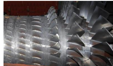
Fig. 1. Photograph of failed compressor rotor.
