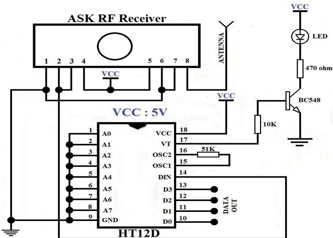
By extending the use of this device the data can be sent to an Arduino which is programmed to behave like a keyboard emulator. The ASCII values of the certain keys desired are set as computer inputs to the respective receiver outputs. For this purpose exclusively Leonardo Arduino is used.
