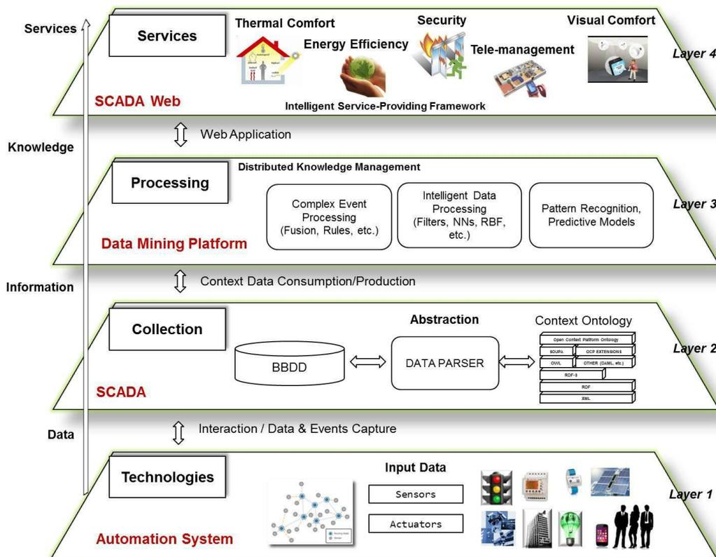
Figure1 IOT Architecture For Smart Building
