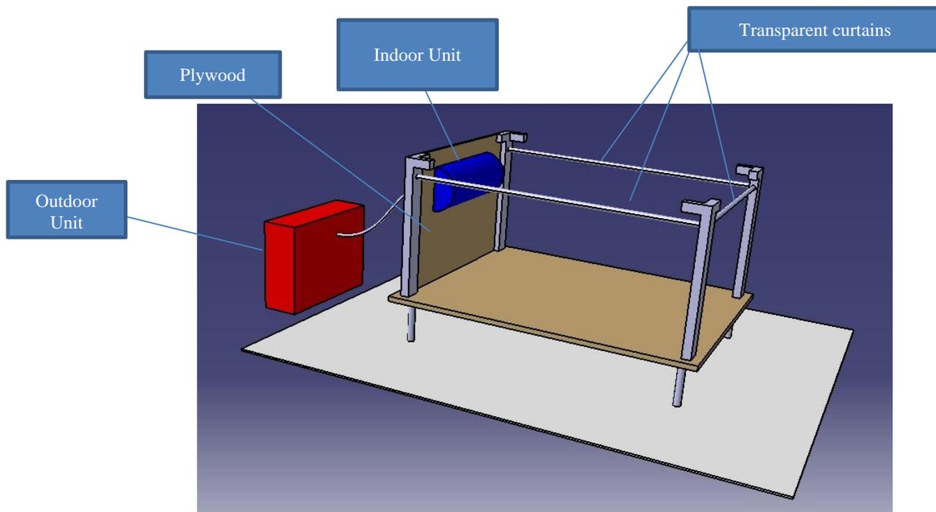
Fig. 1 Proposed Set Up
