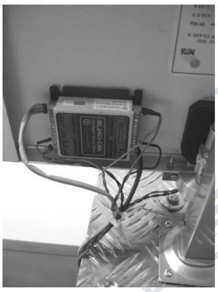
b) Figure 6 Experimental model of a single-axis solar tracking system;
