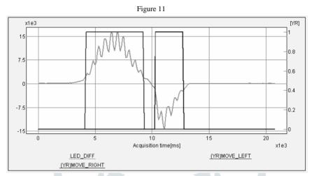
Generation of movement command of the PV panel to the right or to the left when moving a light source from the left to the right in front of the PV panel
