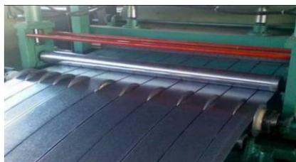
Fig 1. Slitting Operation
