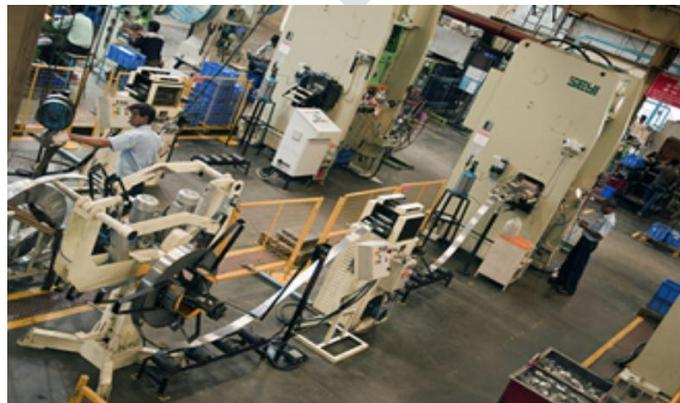
**Fig 8. Automatic sheet flattening machine**
