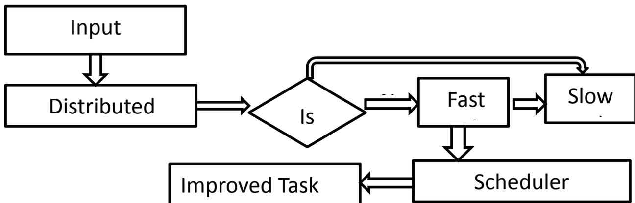
In the Proposed model architecture the two input parameter will be take from workload. The node parameters and job parameter features will be extract and store in the tabular form. Then that data will be give to distributed SVM (support Vector Machine) the SVM is used to predict the straggler with the help of input feature of node parameter and job parameters and identify the which node is slow or fast.
