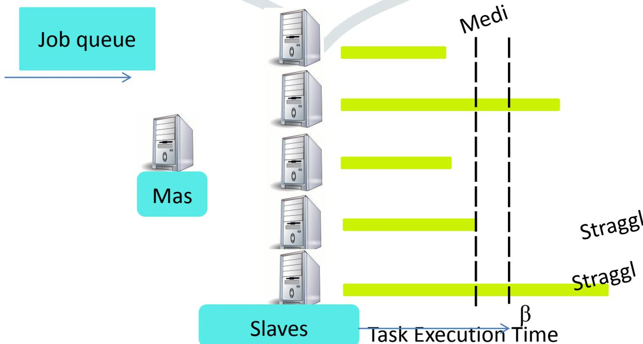
In the above figure the job is given to master machine and the master machine distribute the job into task to slave machine the slave machine has to complete the task in median limit if the slave machine fails to complete the in the time limit then the slave have straggler. So in the figure shown slave machine four and five having straggler because its takes too much time to complete the allocated task.
