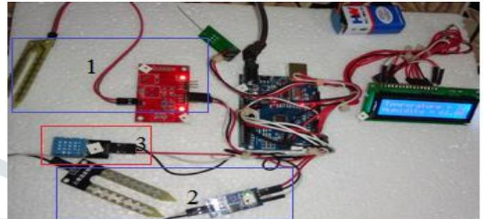
Fig 2 Master unit (1) Soil moisture sensor plant 1, (2) soil moisture sensor plant 2, (3) Humidity and Temperature sensor.
