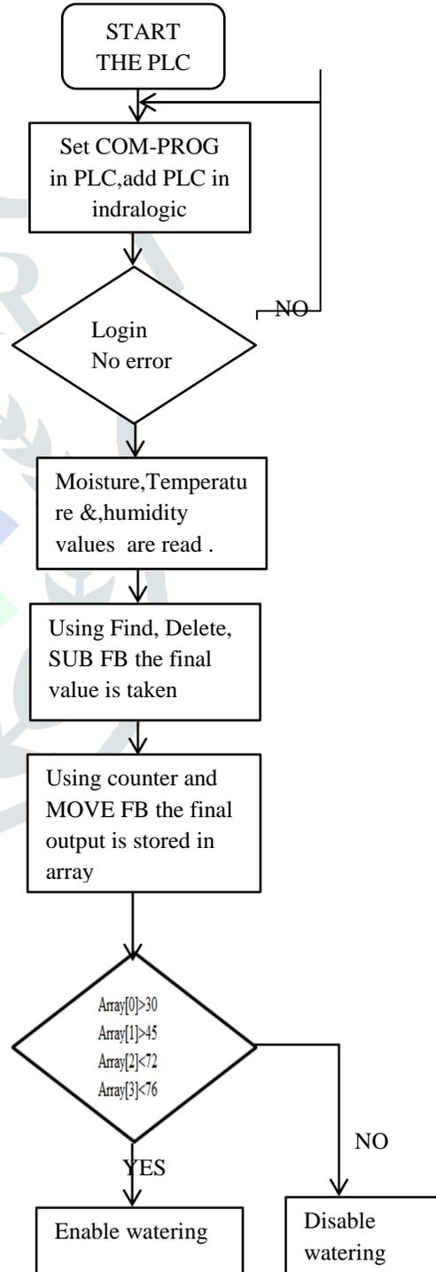
Fig 6 Operational flow chart of PLC
