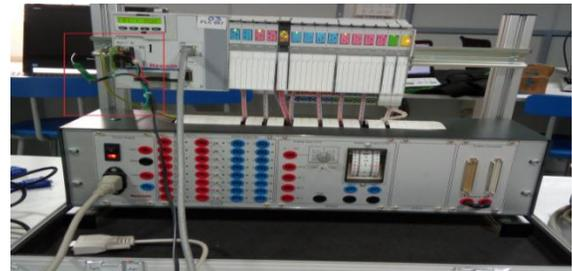
Fig 5 Control unit interfaced with PLC, (1) RF module with RS232
