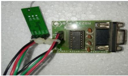
Fig 4 RF module with RS232
