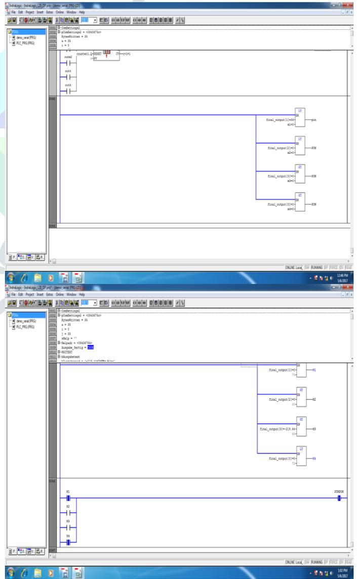
Fig 8 Pump ON and OFF condition displayed in PLC ladder logic
