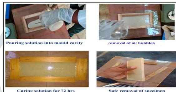
**Fig 3: Specimen preparation**
