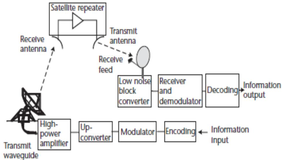
Figure [3]: Critical elements of the satellite link.
