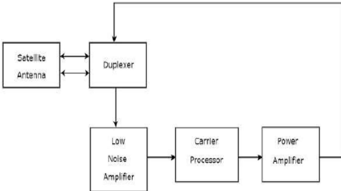
Fig. [1]: The block diagram of transponder
