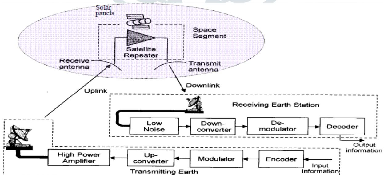
Figure[2]: Basic communications satellite components
