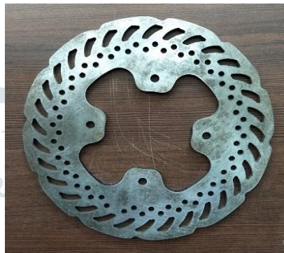
Figure-1: Specimen of Pre-crack Rotor for Test
